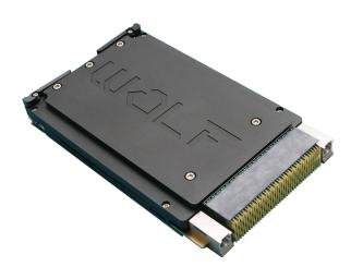
The VPX 3U **WOLF-163S** is a high performance, high port networking board with a Blackwell RTX5000 GPU & 200 Gpbs Ethernet switch supporting 8× 25GBase-KR ports. There is also a 1000BASE-T port. It is available with (163S) & without the GPU (160S).
