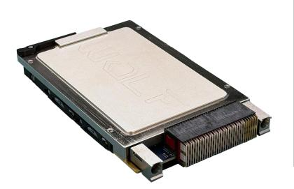
The **WOLF-153L** is a great solution with the Ada RTX5000 GPU and powerful networking ConnectX-7 smartNIC. It features 2× 10GBase-KR ports & 1x 40/100GBase-KR4 port through the CX-7. It can also support Multi-Host & act as the Ethernet switch in larger system networks. It is available in both 14.6.11 & 14.6.13 slot profiles.
