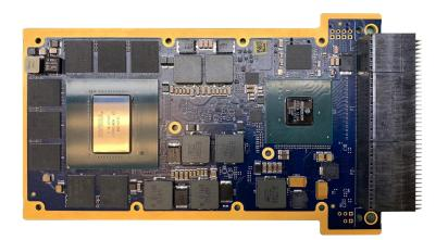
The **WOLF-1538** is an ideal solution for offline GPU processing utilizing the Ada RTX5000 GPU & Gen 4 PCIE switch. It is available in both SOSA 14.6.11-0 & OPENVPX slot profiles. Up to 4x Outputs on P2.
