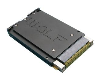
The VPX 3U **WOLF-1570** is a high performance, flexible design with an Ada RTX2000 GPU, Xilinx FGX2 FPGA & PCIe Gen 4 switch. It has up to 4x 12G-SDI Inputs plus 4× 12G-SDI Outputs.
